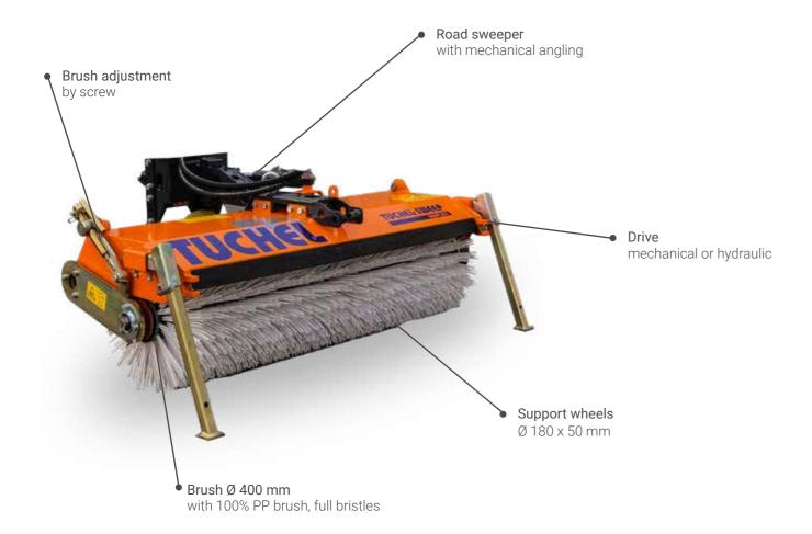
Due to its low dead weight, the SIMPLEX road sweeper is particularly suitable for front-lift systems with low lifting force such as municipal tractors, front mowers, yard loaders or municipal vehicles up to 30 hp.
