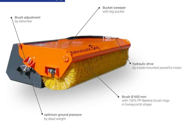
The bucket sweeper is specially designed for your compact / or wheel loader and is equipped with a quick hitch as standard, driven by a powerful hydraulic motor with overpressure relief valve, which is integrated in the roller shaft as standard and thus protected against damage.
